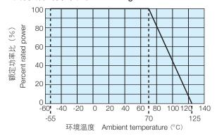
在环境温度70℃以上使用时,应按照上图负荷减轻特性曲线,减小额定功率。 For resistors operated at an ambient temperature of 70°C or above, a power rating shall be derated in accordance with the above derating curve
