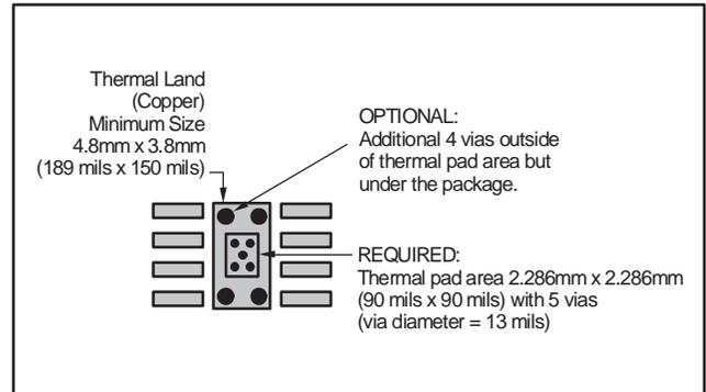
**Figure 11. 8-Pin PowerPAD PCB Etch and Via Pattern**
