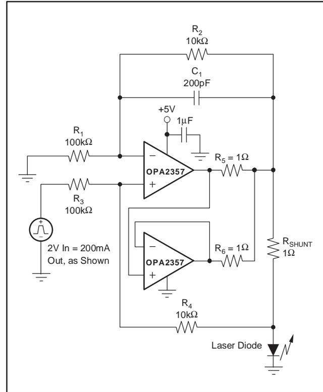
Figure 3. Parallel Operation
