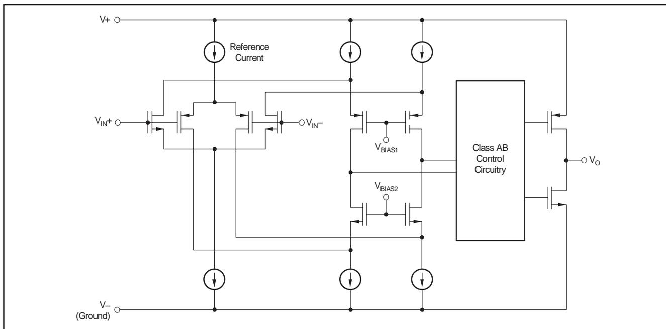
Figure 1. Simplified Schematic
