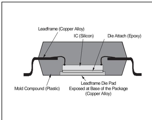
**Figure 10. Section View of a PowerPAD Package**
