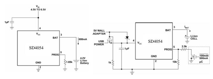
Figure 1. 600mA Single Cell Li-ion Charger
