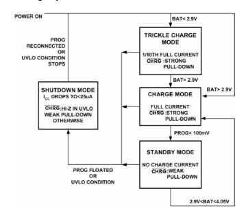
Figure 7. State Diagram of a Typical Charge Cycle
