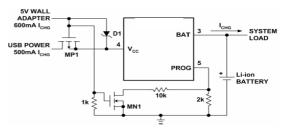
Figure 12. Combining Wall Adapter and USB Power
