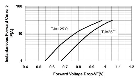
Fig.3-Typical Forward Voltage Drop Characteristics
