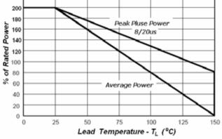
Fig2.Power Derating Curve
