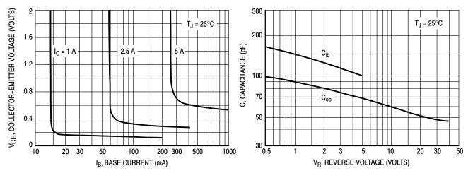
Figure 7. Collector Saturation Region
