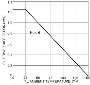
Fig. 11 Power Dissipation vs. Ambient Temperature
