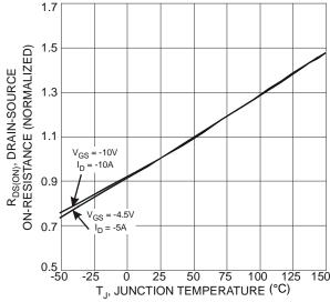
Fig. 8 On-Resistance Variation with Temperature
