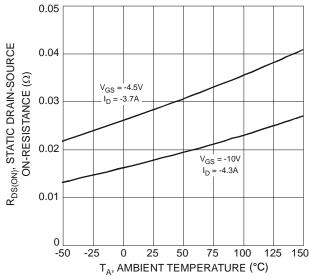
Fig. 4 Static Drain-Source On-Resistance vs. Ambient Temperature
